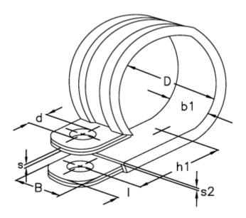
$\begin{array}{lll} \text{b1} & = 25.0 \\ \text{d} & = 8.4 \\ \text{Diameter D} = 39 \\ \text{h1} & = 34.0 \\ \text{I} & = 8.5 \\ \text{s} & = 0.80 \\ \text{s2} & = 2.0 \\ \text{Width B} & = 20 \\ \end{array}$
